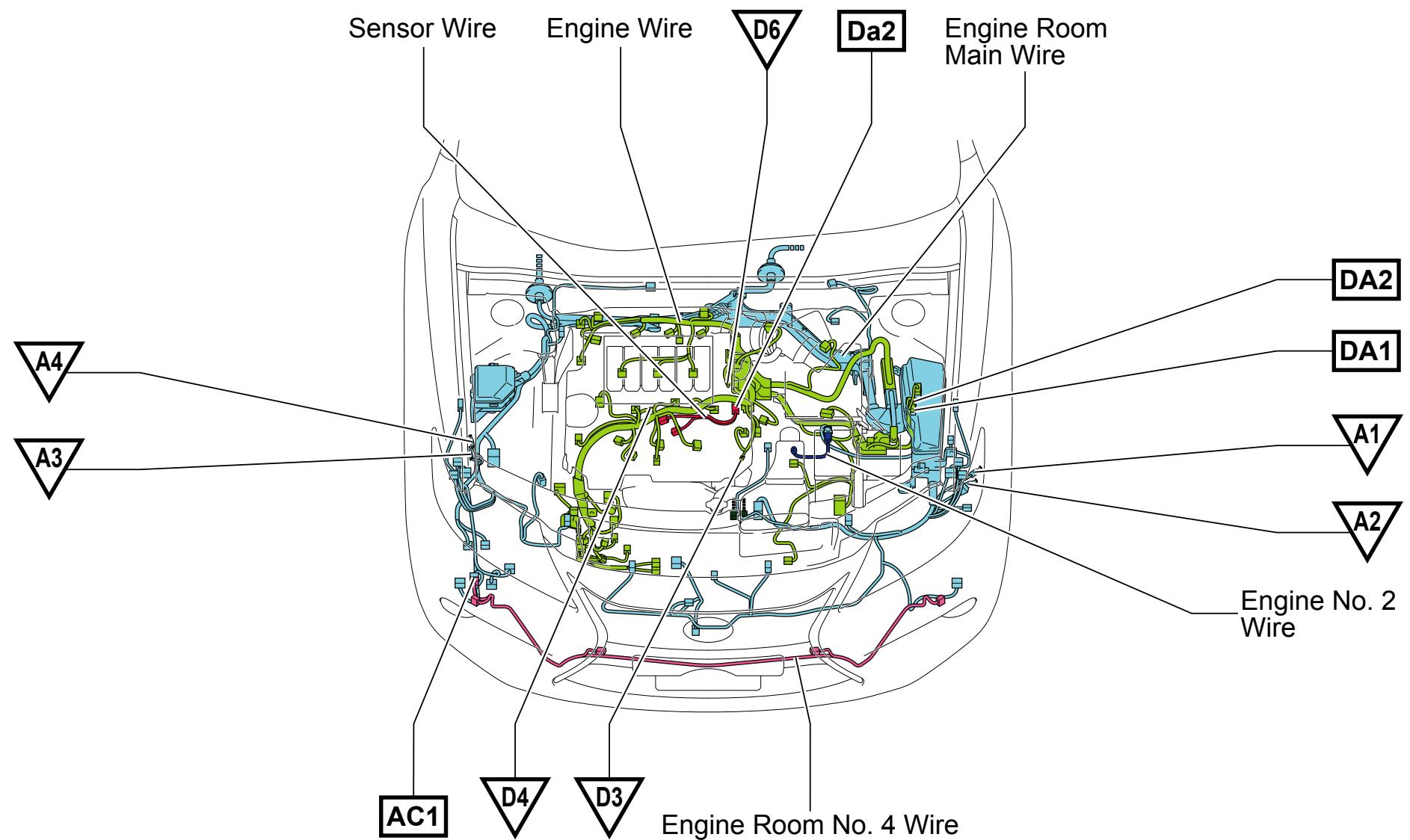
Wire and Wire , Ground Points in Engine Compartment <2GR-FE>
